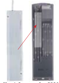
Size 1 Commander GP20 heatsink shown
